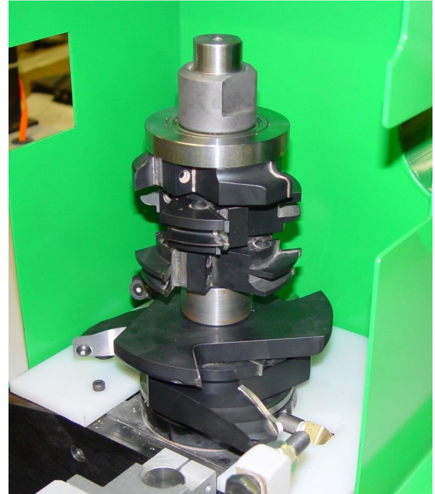
Spindle with cutter stack – not to size.
