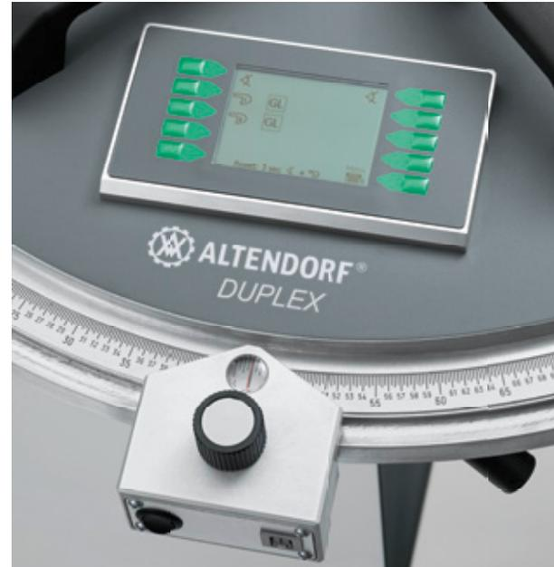
■ **DUPLEX DD:** An exclusive Altendorf development, the DUPLEX DD has been patented worldwide. The high precision DUPLEX DD electronics incorporate automatic length compensation and calculate the distance to the stops as a function of the angle on both sides of the fence and display both figures digitally. Digital angle display and digital length display for adjustment, automatic length compensation. Batteries included. Stops to 1350 mm or 2150 mm.
