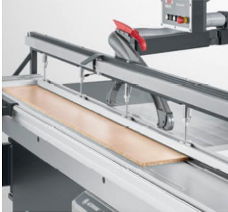
■ **Pneumatic pressure beam:** This is an ideal solution for securely retaining workpieces of up to 80 mm thick, making it particularly useful when working with long and thin materials. It comes in two separately-controlled pieces. A 6 bar pneumatic connection is required.
