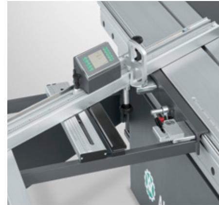
■ **Crosscut-mitre fence with DIGIT L or DIGIT LD:** For 1/10 mm accuracy when setting the length dimension. The display shows all stop settings applied. The central measuring and display unit calibrates the entire system in one operation. Two flip stops with fine adjustment, two batteries and a charger are included.
