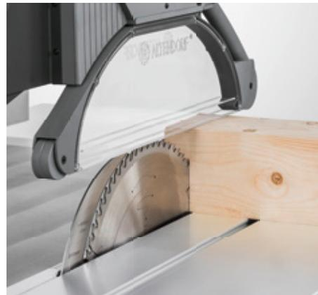
■ **Saw blade protrusion:** The WA 80 saw blade protrusion is 150 mm (saw blade diameter 450 mm). This results in a greater cutting height when crosscutting or square cutting and also when angle cutting with the saw blade tilted.
