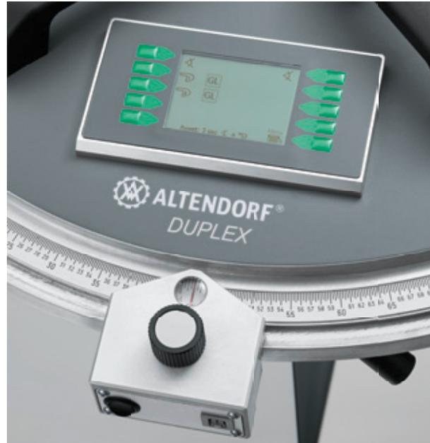
■ **DUPLEX DD:** An exclusive Altendorf development, the DUPLEX DD has been patented worldwide. The high precision DUPLEX DD electronics incorporate automatic length compensation and calculate the distance to the stops as a function of the angle on both sides of the fence and display both figures digitally. Digital angle display and digital length display for adjustment, automatic length compensation. Batteries included. Stops to 1350 mm or 2150 mm.
