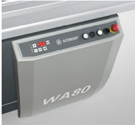
■ **Machine frame control panel:** All functions are easily accessed on the control panel on the machine frame. You can control the rise/fall and tilt of the main saw blade at the touch of a button. The tilt angle is shown on the digital display.
