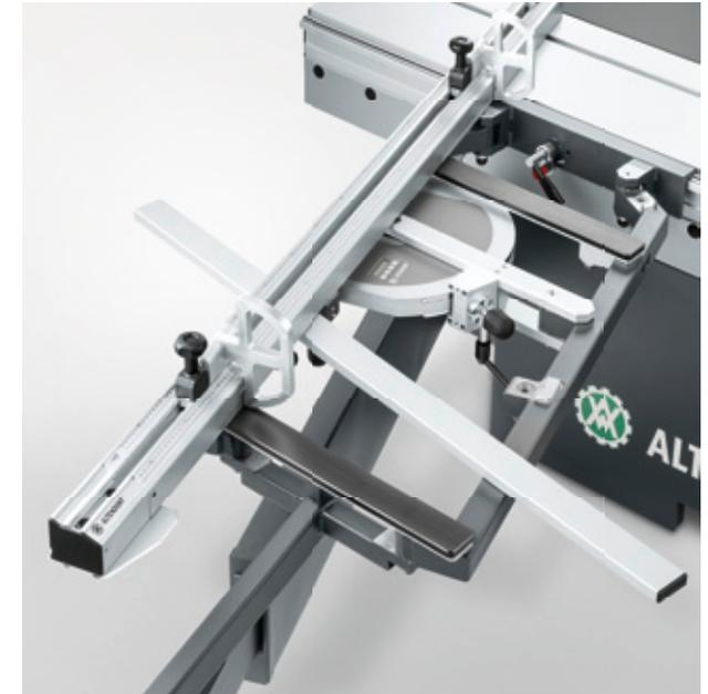
■ **Parallelogram cross slide:** Accurate and wear-free, this system features a robust 90° locking mechanism that ensures the right-angle position is absolutely reproducible. The fence can be angled by up to 47° in either direction. The integrated digital display shows the angle with an accuracy of 1/100° for optimal precision. Also included is length compensation, which is simply taken from a scale when the fence is angled. Two flip stops are included. Stops to 3500 mm.
