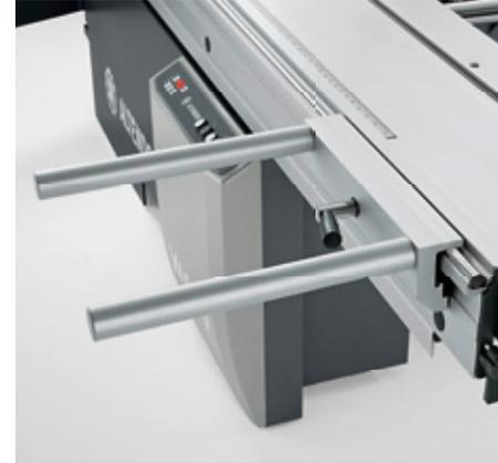
■ **STEG:** Enlarges support area (width: 400 mm) for wider workpieces. Makes it much easier to size large panels.
