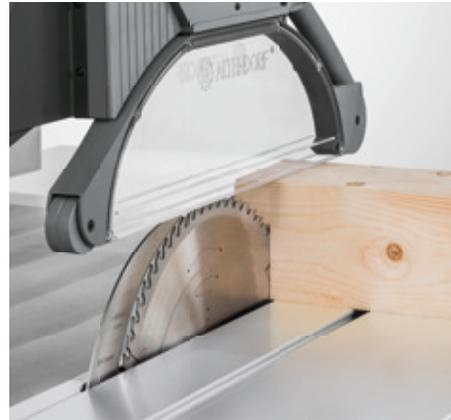
■ **Saw blade protrusion:** The WA 80 saw blade protrusion is 150 mm (saw blade diameter 450 mm). This results in a greater cutting height when crosscutting or square cutting and also when angle cutting with the saw blade tilted.
