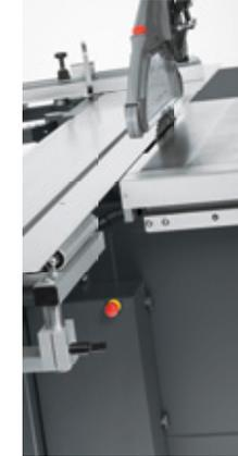
■ **Front support roller:** The 300 mm-wide infeed support roller is particularly useful when cutting longer workpieces against the rip fence. It folds away under the sliding table (minimum length 3 000 mm) when not required.
