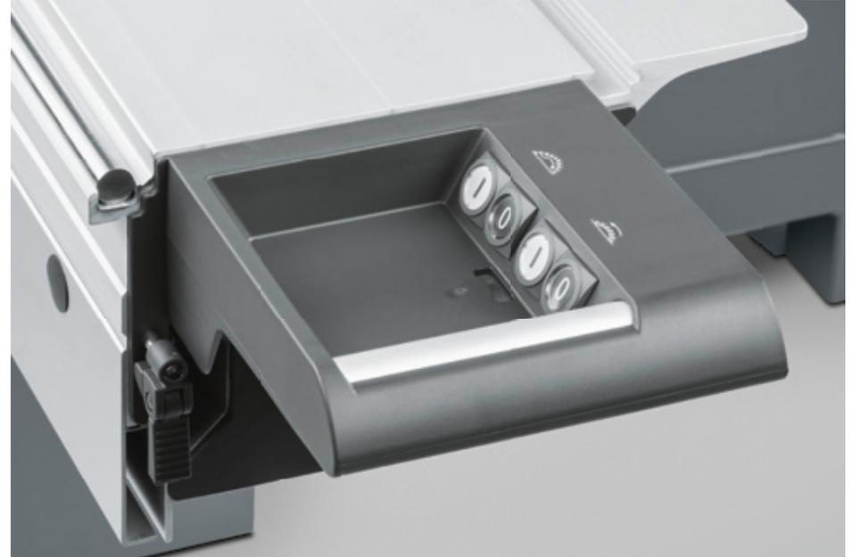
■ **On/off switches on sliding table:** The practical option. The on/off switches are always right where you need them, at the end of the sliding table. The four keys switch both the main and scoring blades on and off. This option allows you to load a large workpiece before switching the machine on, thus improving safety and convenience. The keys can be operated without you having to switch specially between the machine operating panel and the sliding table switches.
