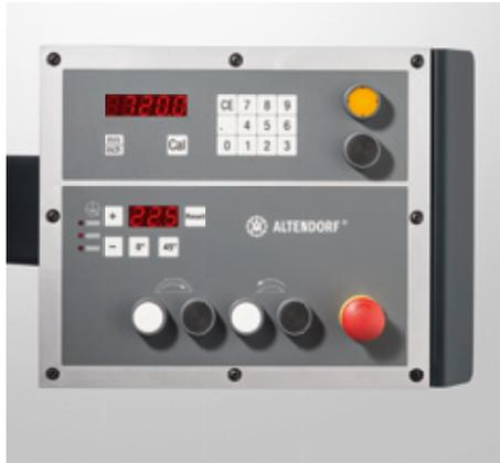
■ **Eye-level operating panel:** All major control functions are always visible. The panel pivots into the most convenient position and is accessible from both sides of the machine. Adjustment of both the saw blade and the rip fence are motorised.
