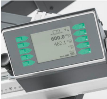
■ **Crosscut fence with DIGIT L:** For 1/10 mm accuracy when setting the length dimension. The display shows all stop settings at the same time, and allows calibration of all stops in one operation. Two flip stops with fine adjustment, two batteries and a charger are included.
