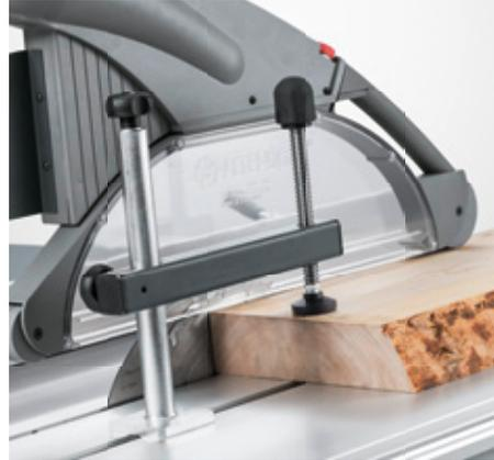
■ **Manual quick-action clamp:** The manual quick-action clamp can be positioned on the sliding table easily and is equally easy to fix in place, ensuring the workpiece is reliably retained on the table and against the crosscut fence. It has a clamping height of up to 200 mm and provides extra safety at very little extra cost.
