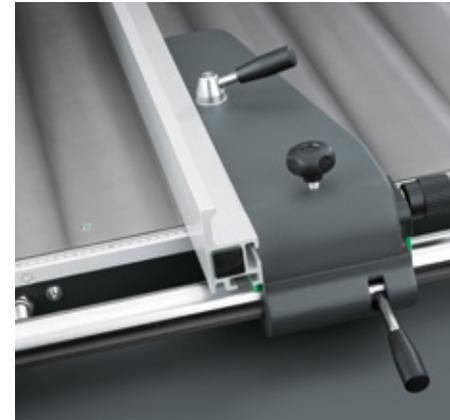
■ **Rip fence with manual fine adjustment:** Setting the fence is easy; the precision fine adjustment makes for great accuracy. The hard chrome-plated round bar system ensures the fence moves smoothly. The rip fence drops down clear of the machine table level to free up extra space for dividing large panels. Available cutting widths: 800 mm, 1000 mm or 1300 mm.
