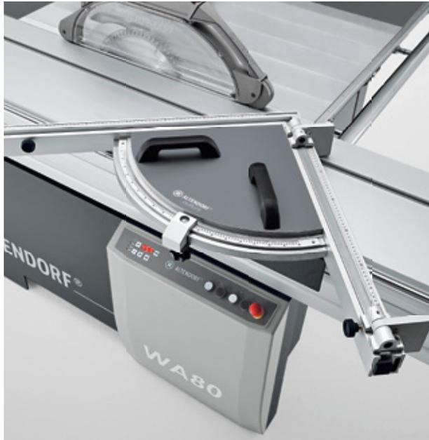
■ **DUPLEX double-sided mitre fence:** DUPLEX fences make it possible to cut any angle between 0 and 90° very quickly and exactly. Set the DUPLEX to 45° and a mitre cut can be made on both sides of the workpiece without resetting the two fences. Dimensions are set using a magnifier, a measuring scale and a length compensation scale. All DUPLEX fences can be positioned anywhere along the entire length of the sliding table.
