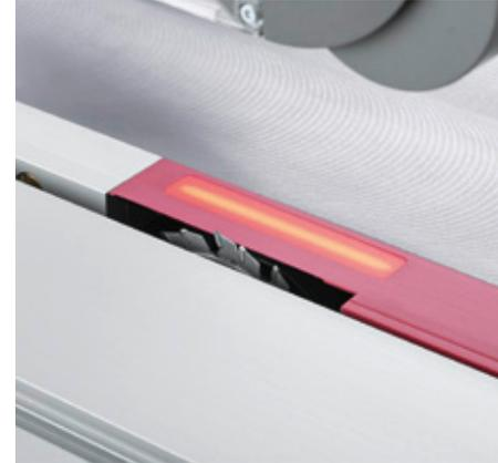
■ **LED illumination:** Particularly energy-efficient LEDs render the danger area around the scorer highly visible.
