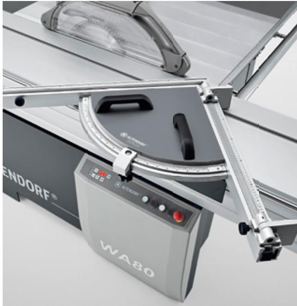
■ **DUPLEX double-sided mitre fence:** DUPLEX fences make it possible to cut any angle between 0 and 90° very quickly and exactly. Set the DUPLEX to 45° and a mitre cut can be made on both sides of the workpiece without resetting the two fences. Dimensions are set using a magnifier, a measuring scale and a length compensation scale. All DUPLEX fences can be positioned anywhere along the entire length of the sliding table.
