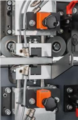
Surface scraper with dual-tracing
