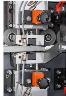
Surface scraper with dual-tracing (optional)
