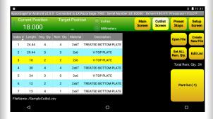
Create your cutlists at the machine or email a cutlist over a WiFi network. The Android has tremendous storage capacity, so you are not limited to saving only small cut lists. Cutlists can also be restored to original quantities after use or even multiplied if you want to make several "kits" of parts at once.
