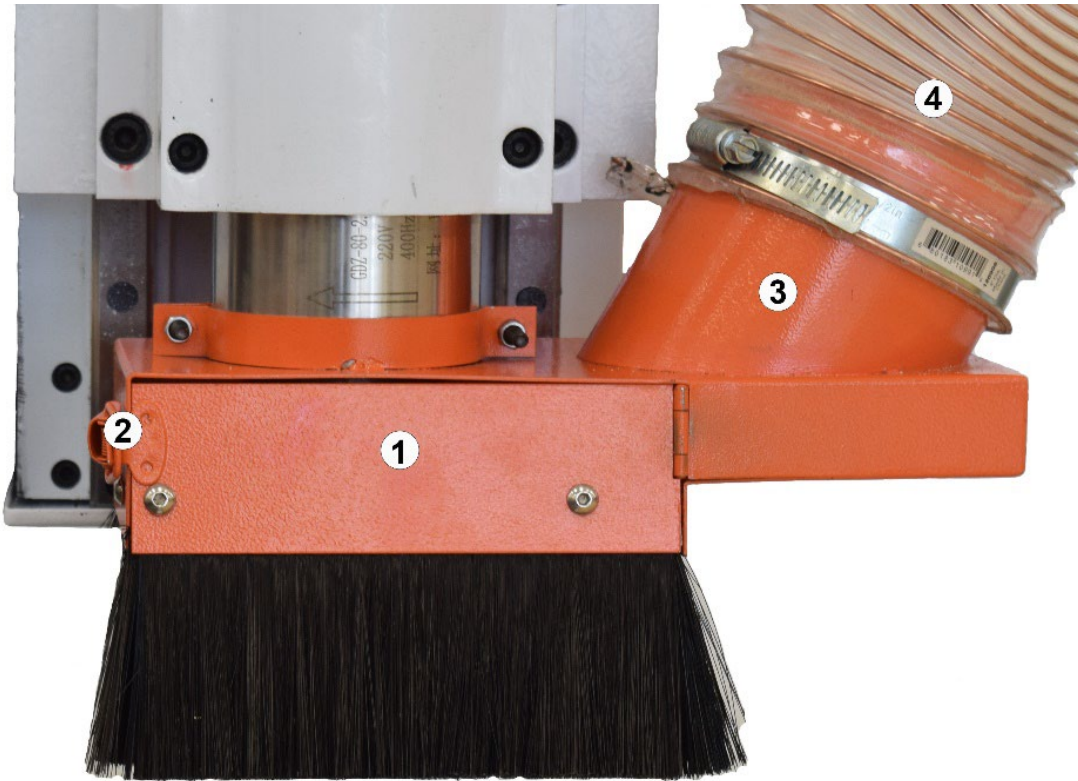
Figure 5-5: Dust Collection Components
