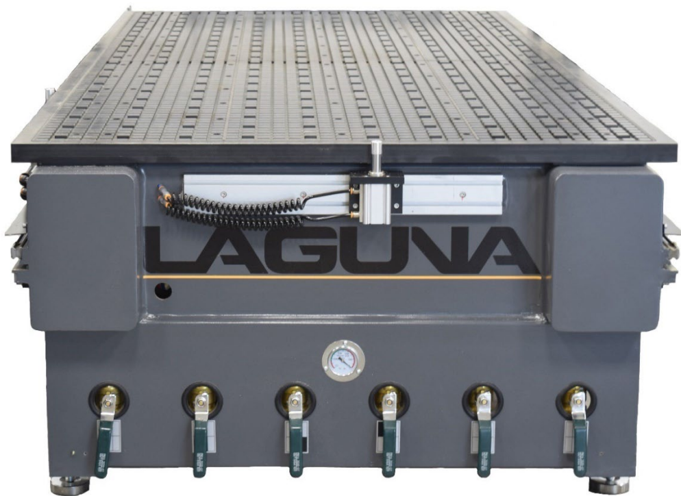
Figure 5-3: Vacuum Table and Control Levers
