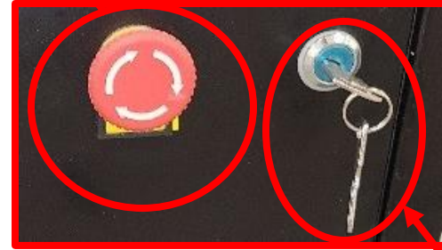
Conveyor Manual Switch- Used to move conveyor belt when Machine is "Manual Mode".
