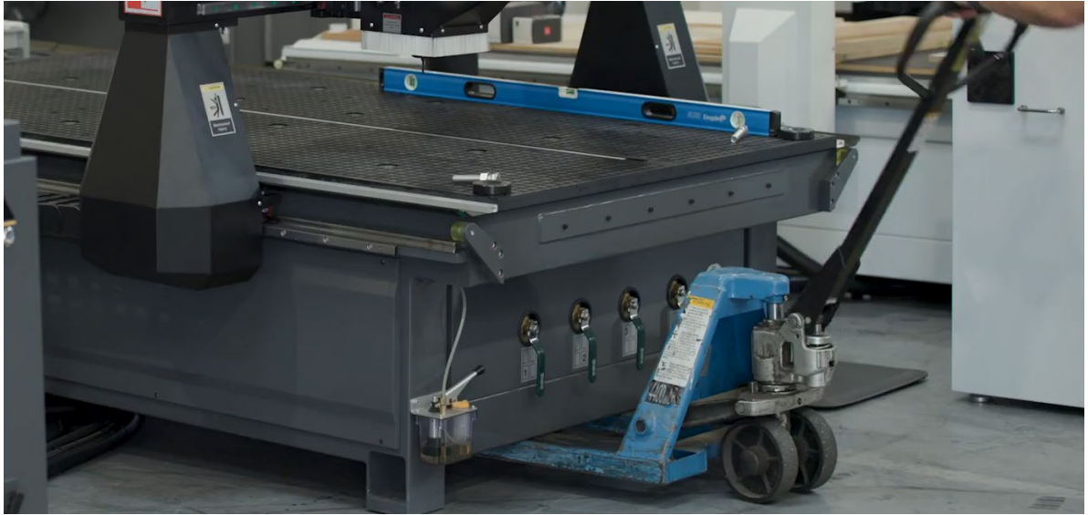
Figure 9–1: Pallet Jack Lifting the Machine
