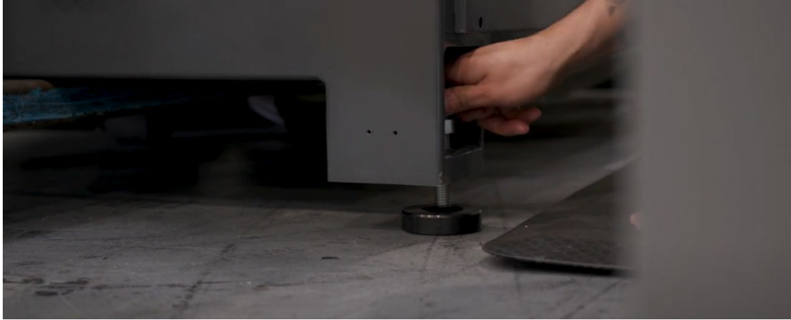
Figure 9–3: Inserting and Turning Bolt Against the Metal Foot
