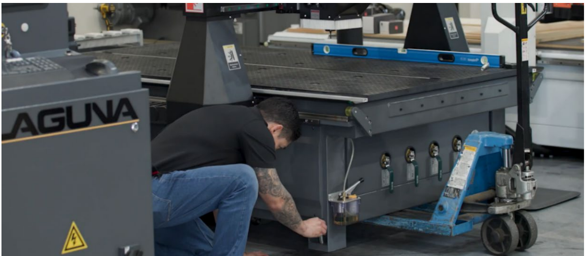
Figure 9–2: Aligning the Metal Feet
