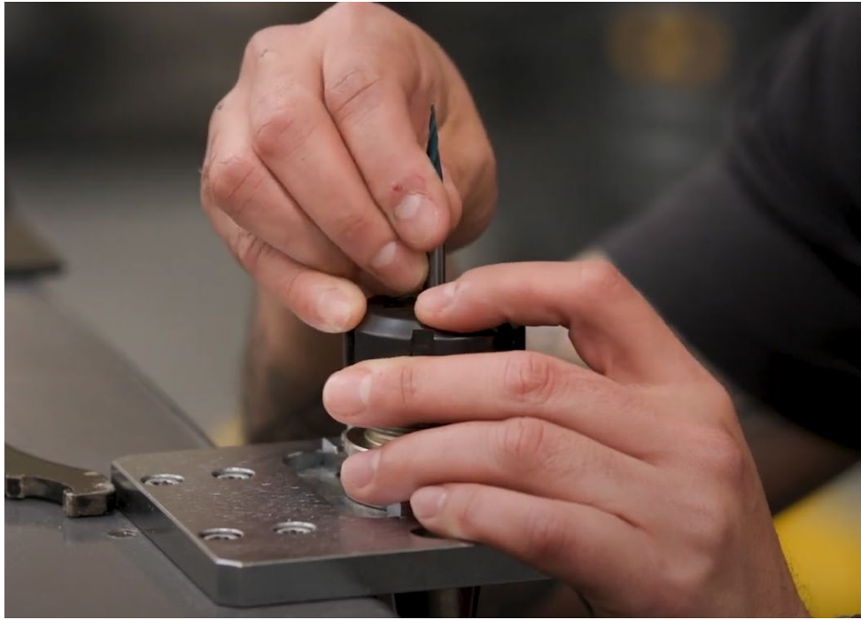
Figure 16–4: Placing Bit into the Collet
