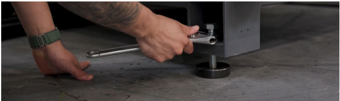
Figure 9–4: Using a Crescent Wrench to Adjust and Tighten the Bolt/Nut Combo
