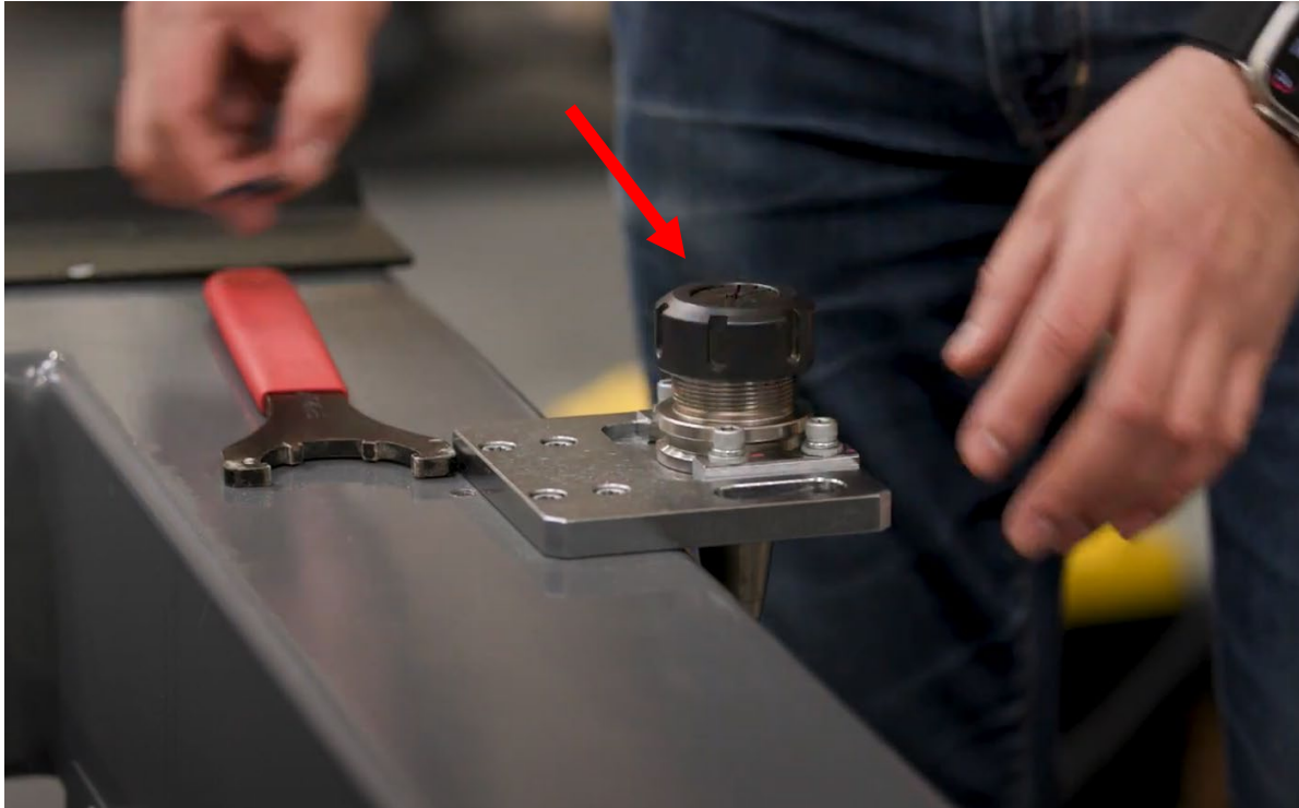
Figure 16-3: Spindle Nut on Cone
