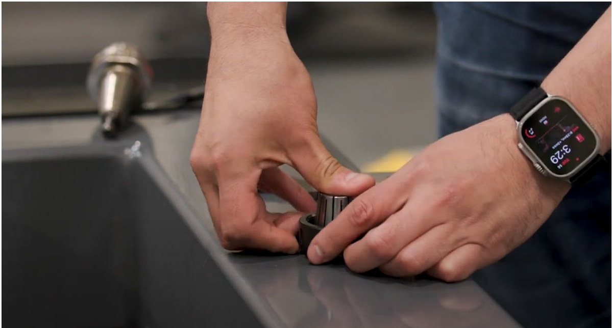
Figure 16–1: Pressing Collet into Spindle Nut
